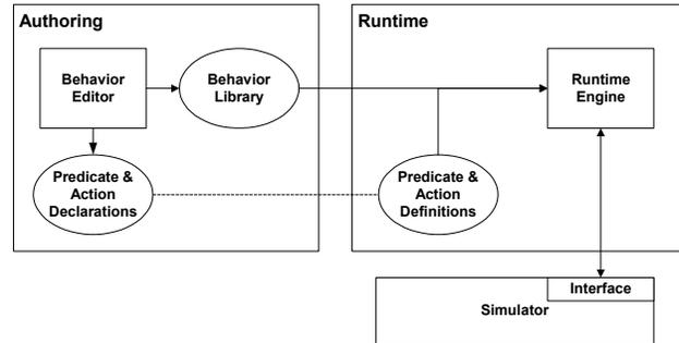
Figure 3. Components of Authoring System
