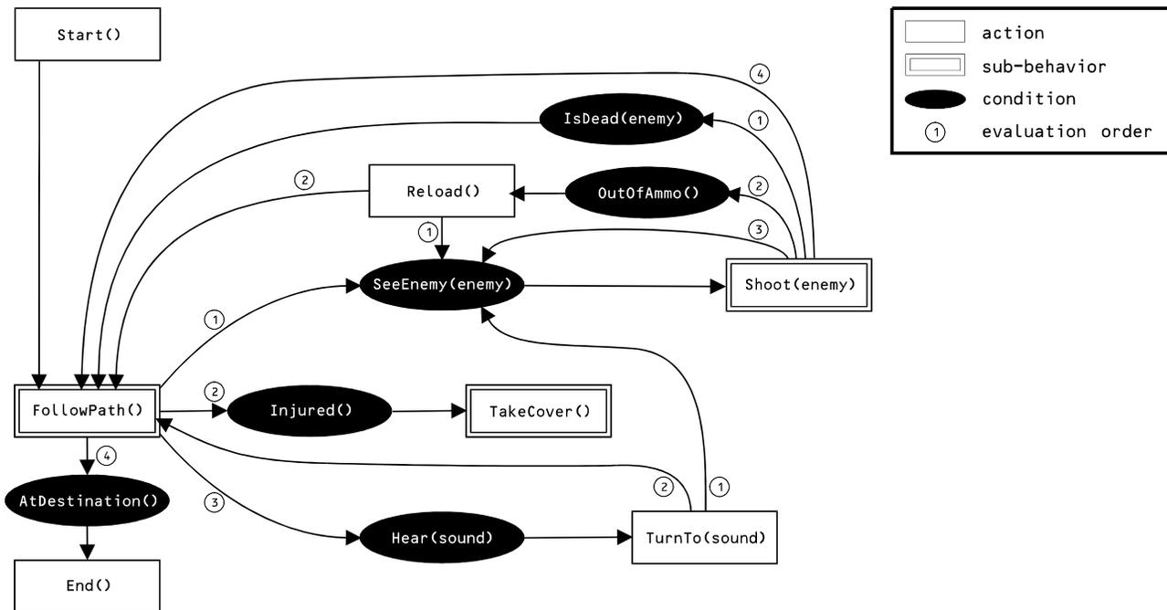
**Figure 1.** The *CombatPatrol* Behavior Transition Network
